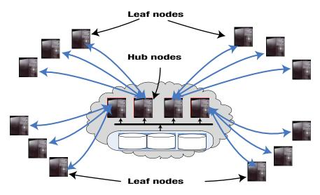
Figure 4-1. Hub-and-spoke topology of Oracle Flex Clusters
