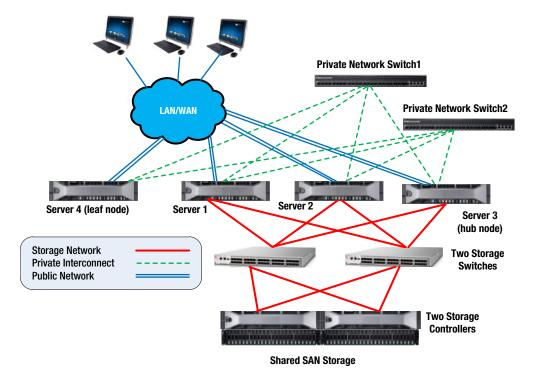
Figure 1-2. Oracle RAC hardware architecture
