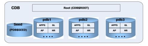
Figure 4-8. Architecture of CDB with PDBs
