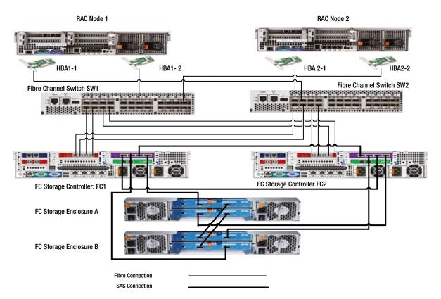
Figure 5-4. FC switch fabric topology
